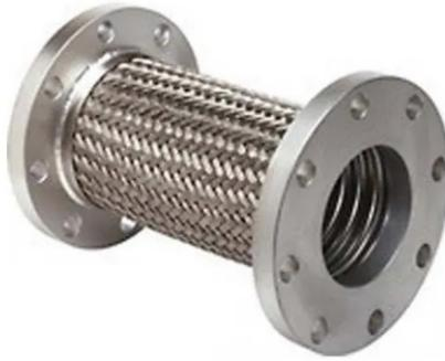
Ordinary flexible metal hoses can fail to operate properly when subjected to high pressures; adding a flexible restraint, such as a metal braid, allows the hose to adequately withstand the specified internal pressure and prevent elongation. The woven metal braid is designed to fit over the metal hose, and to be strong enough to withstand elongation up to the full pressure rating of the hose.
